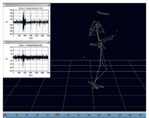
Figure 24. Motion captures of an individual walking on the treadmill and holding a mobile device to assist navigation performance. The positions of the reflective markers attached to the body of the participant are captured by several infrared cameras and postprocessed according to biomechanical models to arrive at a dynamic visualization of the participant's movements. The two boxes depict a simultaneously recorded EMG signal from the right arm.
