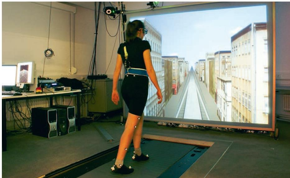
Figure 23. A young adult walking on the treadmill through a virtual world. Reflective markers and a system of infrared cameras allow for the analysis of gait characteristics and for the adaptive regulation of treadmill speed.
