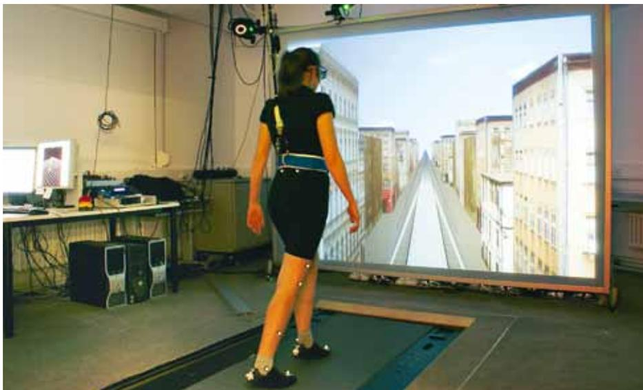
Figure 20. A young participant walking on the treadmill through a virtual world. Reflective markers and a system of infrared cameras enable gait characteristics to be analyzed and treadmill speed to be adaptively regulated.
