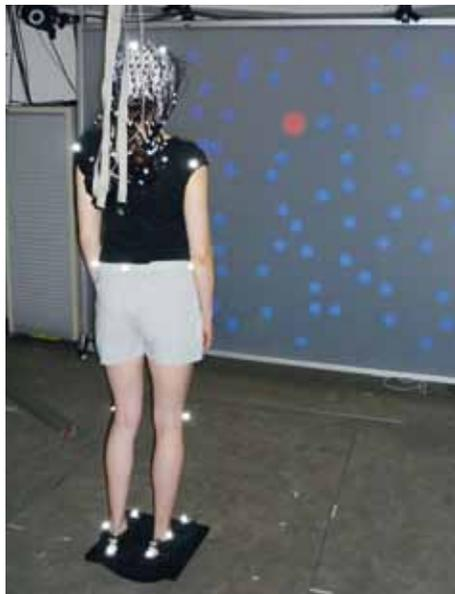
**Figure 21.** A young adult fitted with EEG sensors and reflective motion capture markers participating in an experiment investigating the neural correlates of the visual stabilization of balance. The red and blue dots presented on the screen flickered at different frequencies to analyze the entrainment of cortical activity to central and peripheral visual stimuli under various conditions of postural stability.
